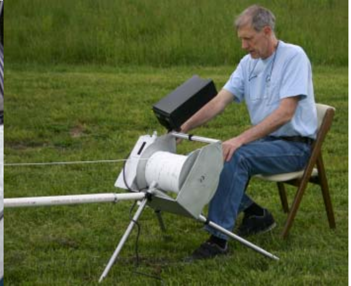
The Deluxe GeoVISION™ system in field use. Note the push pole attached to the front to provide additional stability in deep boreholes.
